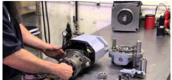
Hydraulic Pump Repair
